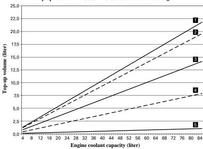
In case of expansion tank at normal level, this quantity is to be drained from the cooling system.
