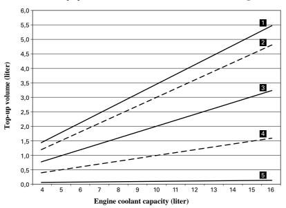
In case of expansion tank at low level, this quantity is to be filled without draining from the cooling system.
