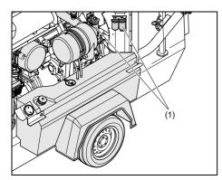
Replacing the filter element
