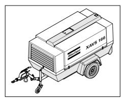
The compressors type XAHS 146 Dd, XATS 156 Dd, XA(S) 186 Dd, XAVS 166 Dd and XAHS 186 Dd are silenced, single-stage, oil-injected screw compressors, built for a nominal effective working pressure, ranging from 7 bar (102 psi) up to 12 bar (175 psi) (see chapter **Technical specifications**).
