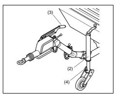
Adjustable towbar with jockey wheel and brakes
