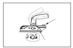
Check the coupling head fastenings
