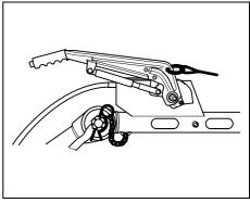
Hand brake lever downward - brake not operated
